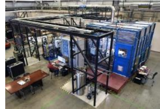
25 kW high-temperature electrolysis @ INL Energy Systems Laboratory
